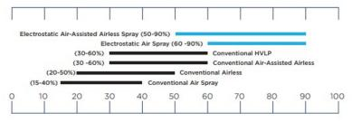
This chart represents typical direct charge equipment transfer efficiencies, but not every installation. Conditions may vary due to material and application.
